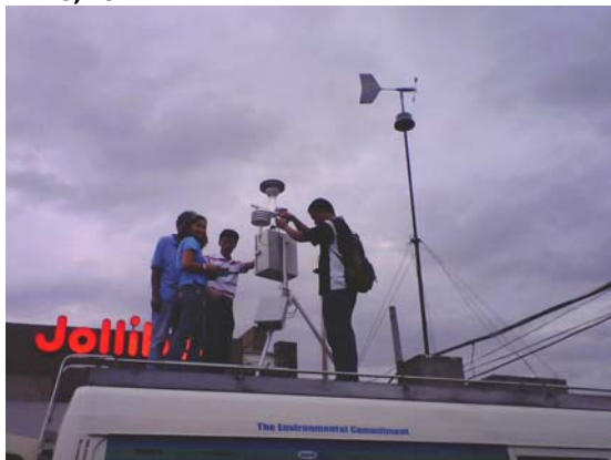
Set-up of Horiba Air Quality Monitoring System (CO, NO 2 ) and E-BAM (PM 10 )
